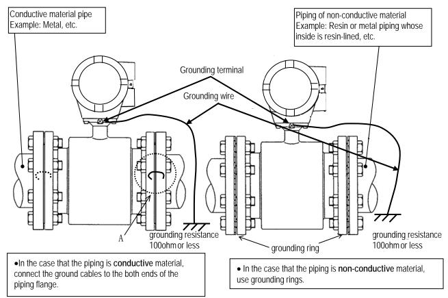
Figure 4.12 Grounding the GF630/LF600F and GF630/LF610F Type
